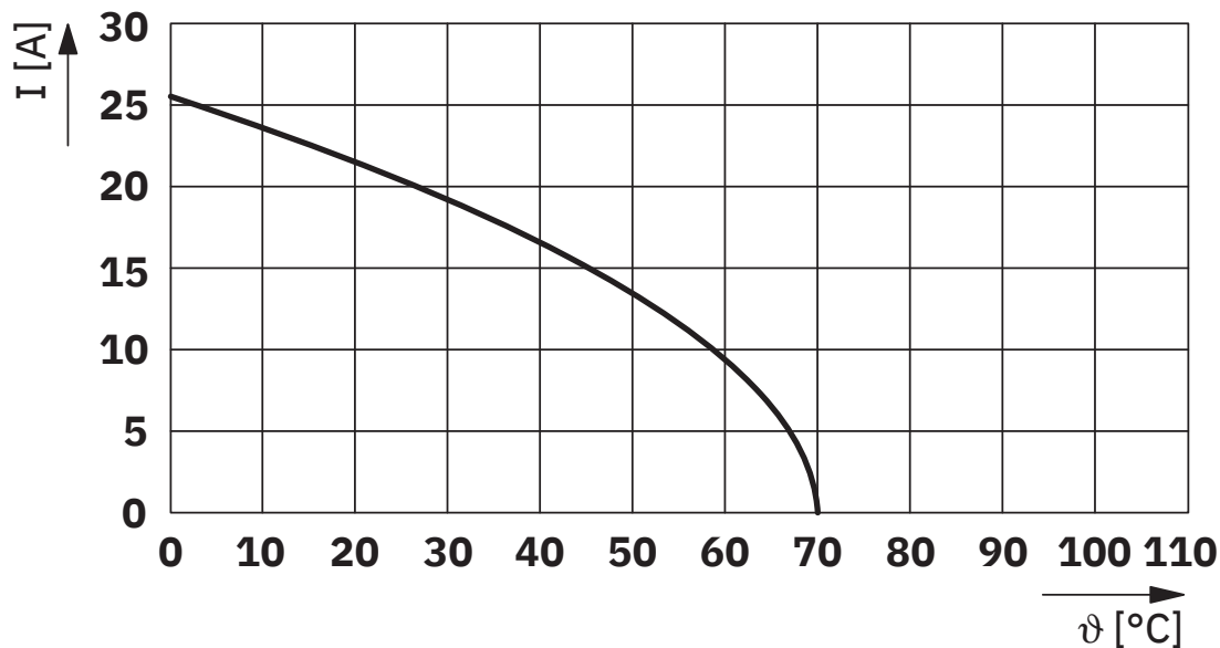
Derating diagram for cable, flexible installation
